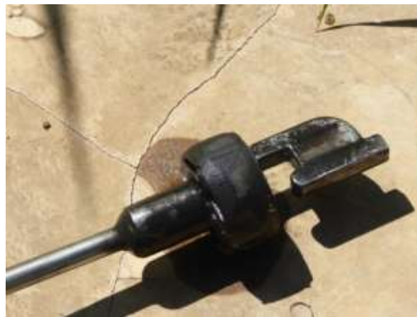
Figure 11. Black residue due to corrosion by saline water at 18. Kabira
